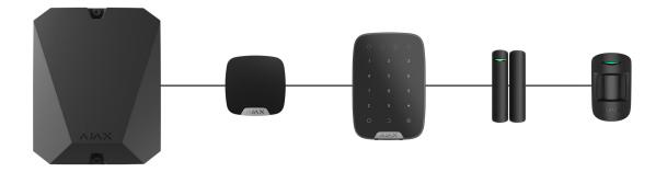
For the **Beam** (**Radial**) topology, be sure to install a 120 Ohm terminating resistor at the end of the line (included in the hub complete set). The terminating resistor is connected to the signal terminals of the last detector on the line.
