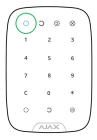
KeyPad Fibra can report the current security mode, button pressings, malfunctions, and other conditions with LED indication and a sound signal.
